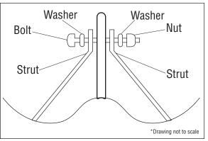
$\square$  14. Repeat steps 10 through 13 for the remaining top wire. Once both wires are set to length, use a 4-40 x 5/8-inch button head cap screw, two #4 washers and a 4-40 lock nut to secure the top wires to the fin.
