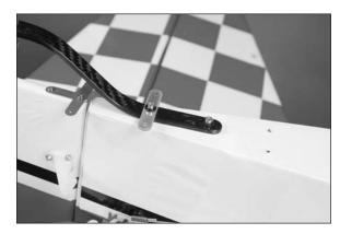
☐ 9. Connect the arm from the tail wheel to the tiller arm using two tail wheel steering springs. Make a loop on each end of the spring with needle nose pliers. Use care when bending the springs so the tail wheel is aligned with the rudder. Cut the excess spring using side cutters.
