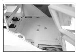
$\square$  5. Install the seat by attaching the magnet from the seat to those in the painted plywood plate.
