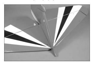
☐ 5. Remove the packaging from the tail of the fuselage. Place the assembly on the fuselage. The fin will fit into the slot along the top of the fuselage.
