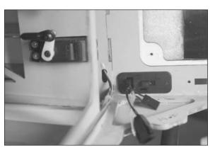
$\square$  2. Follow the procedure as described in your radio manual for binding the receiver and transmitter. Check the operation of the rudder, elevator and throttle servos using the radio system.
