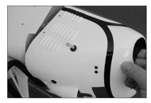
☐ 4. Guide the cowl into position. The holes in the cowl will line up with the holes in the fuselage. Use four 4-40 x 1/2-inch button head cap screws and four #4 nylon washers to secure the cowl. Tighten the screws using a 5/64-inch hex wrench.
