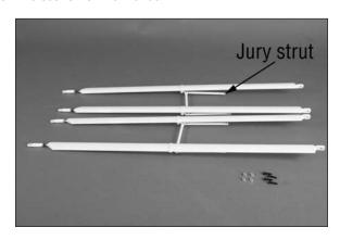
$\square$  2. When installing the wing struts, the airfoil of the strut will match that of the wing when the jury struts are facing toward the fittings on the wing. Use two 4-40 x 1/2-inch button head cap screws and two 4-40 lock nuts to secure the struts to the fittings. Use a 5/64-inch hex wrench and 1/4-inch nut driver to tighten the hardware.
