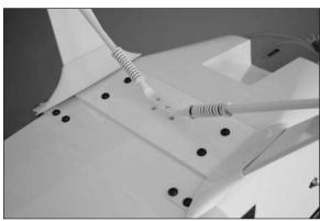
**Hint**: A machined hex wrench is helpful to allow the bolts to be tightened and not strip the head of the bolt.
