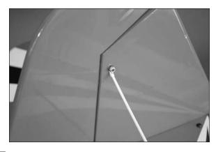
☐ 15. Check the alignment of the fin to the stabilizer to make sure they are perpendicular to each other. Also check the alignment between the rudder and fuselage. If not, loosen the hardware slightly to adjust the alignment.
