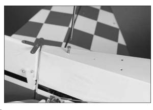
$\square$  7. Place 2–3 drops of thin CA in each hole to harden the surrounding wood. This will keep the screws from vibrating loose in flight.
