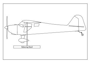
☐ 3. You should find the CG to be very close with the components installed as shown in this manual. If the nose of your aircraft hangs low, add weight to the rear of the aircraft. If the tail hangs low, add weight to the nose of the aircraft. Stick-on weights are available at your local hobby store and work well for this purpose.
