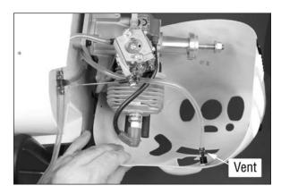
$\square$  3. Remove the plug for the fill line from the cowl. While guiding the cowl on the fuselage, guide the line from the T-fitting through the fill line in the cowl.
