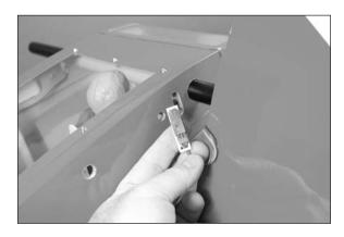
□□ 4. Slide the wing tight against the fuselage.
