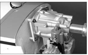
$\square$  3. Use side cutters to cut the tie-wrap holding the ignition ground leads and fuel tubing together.
