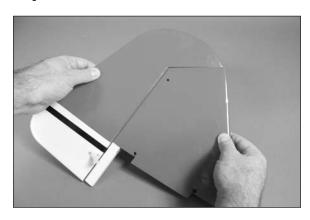
$\square$  3. Separate the stabilizer halves. Slide the pins and one stabilizer half into the holes in the fin as shown.
