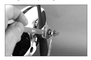
□ 9. The spinner can now be attached using the screw provided and a 4mm hex wrench. Make sure the spinner does not contact the propeller when it is installed.
