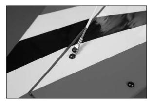
$\square$  13. Adjust the length of the top wire so it just contacts the fin when positioned so the fin is 90 degrees to the stabilizer.
