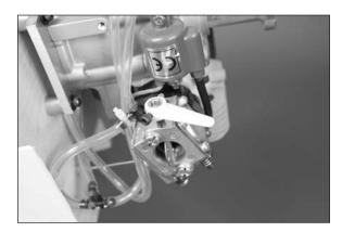
☐ 11. Connect the ball link to the carburetor arm. The pushrod should slide easily as it is not connected to the throttle servo. Use needle nose pliers to snap the ball link on the ball.
