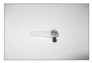
☐ 10. Install the included nylon choke arm on the brass shaft of the carburetor. Be sure the arm can rotate fully and does not hit the engine cylinder. Access the arm by reaching through the front cowl opening inlet with your finger or a small piece of wire with a hook on the end (not supplied). Tighten the screw in the arm using a 7/64-inch hex wrench.
