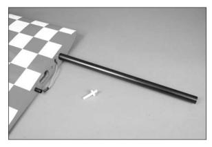
$\square \square$  2. Remove the pins, keepers and silicone tubing from the fitting on the fuselage.
