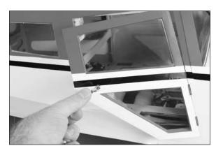
☐ 2. Connect the charger lead to the connection at the charge jack. The model includes a 2700mAh 5-cell Nickel-Metal Hydride (Ni-MH) battery. Be sure and use a good quality charger. We recommend to cycle the receiver battery 2–3 times prior to flying.
