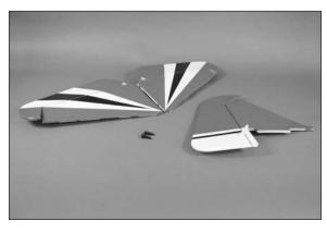
☐ 2. Check that the hinges are glued securely by gently separating the control surface from the fixed surface. If any loose hinges are found, apply thin CA to both sides of the hinge. Allow the CA to soak into the hinge before checking them again.
