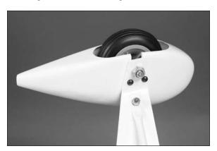
☐ 5. With the landing gear fairing as close to the fuselage as possible, apply a small amount of silicone adhesive to the plywood inside the landing gear fairing. Slide the fairing tight against the fuselage and use low-tack tape to hold it in position until the adhesive cures. Gluing the fairing to the gear will allow the gear to be removed without damaging the fuselage.
