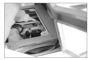
☐ 4. Secure the painted plywood plate in the fuselage using four 2mm x 10mm washer head wood screws and a #1 Phillips screwdriver. Note that the plate will have the single magnet to the front of the fuselage as shown.
