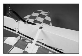
□□ 4. Use a 4-40 x 5/8-inch button head cap screw, #4 washer and 4-40 lock nut to attach the strut to the forward hole of the stabilizer. Place the washer on the screw before passing it through the strut so it is between the head of the screw and the stabilizer. Once everything is positioned, use a 1/4-inch nut driver and a 5/64-inch hex wrench to tighten the hardware. Use care not to over-tighten the hardware and damage the underlying structure.
