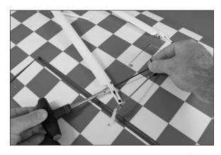
**Note**: Do not over-tighten the hardware that secures the wing struts to the fittings so the struts can be folded in for transport.
