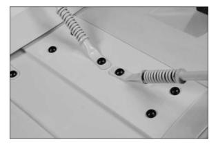
$\square$  4. Attach the wheel pants to the landing gear using four 4-40 x 1/2-inch button head cap screws and four #4 washers. Tighten the screws using 5/64-inch hex wrench.
