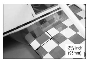
☐ 2. When balancing your model, make sure it is assembled and ready for flight with the fuel tank empty. Support the plane upright at the marks made on the wing with your fingers or a commercially available balancing stand. This is the correct balance point for your model.
