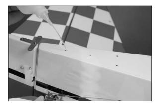
$\square$  8. Attach the tail wheel assembly and the aluminum spreader tab on the fuselage using two 3mm x 15mm socket head wood screws and two 3mm washers. Tighten the screws using a 2.5mm hex wrench.
