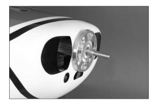
Important: Always balance your propeller. An unbalanced propeller can cause vibrations to be transmitted into the airframe, which could damage the airframe or other components as well as produce unwanted flight characteristics.
