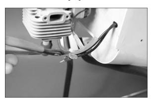
☐ 4. Check that the ignition switch is in the off position before connecting the leads to the engine in the following step. This will prevent accidentally starting the engine if the propeller shaft is rotated.
