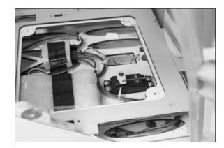
☐ 13. Check the operation of the throttle using the radio system. It may be necessary to change the travel adjust at the radio to prevent the servo from binding at high- and low-throttle. Make sure when the throttle is at idle the butterfly in the carburetor is closed.
