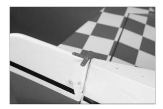
☐ 6. Use a 2.5mm hex wrench to thread a 3mm x 15mm socket head wood screw into the holes in the bottom of the fuselage for mounting the tail wheel assembly. This will cut threads in the surrounding wood. Remove the screws from the holes.
