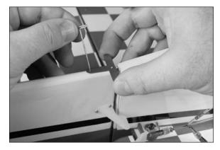
☐ 3. Use a 2mm x 15mm Phillips wood screw and a #1 Phillips screwdriver to make the holes for the two mounting screws in the bottom of the rudder.
