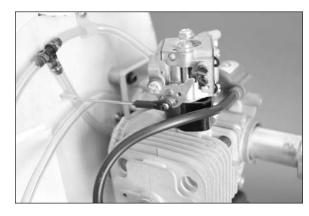
**Hint**: Remove the idle limit setscrew as you will adjust the idle from your transmitter using the throttle trim.
