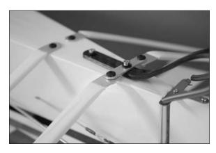
$\square \square$  7. Use needle nose pliers to bend the brass tab at about a 30-degree angle.
