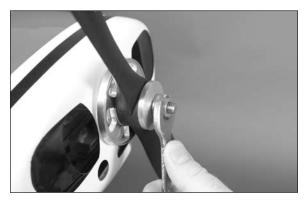
$\square$  8. Thread the spinner adapter on the engine shaft. While holding the larger nut with a 1/2-inch wrench, use a 14mm wrench to tighten the adapter nut against the first nut.
