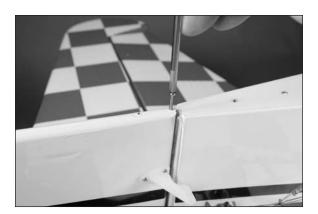
☐ 4. Remove the screw and place 2–3 drops of thin CA in each hole to harden the surrounding wood. This will keep the screws from vibrating loose.
